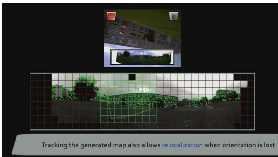
Figure 23: The panorama tracker creates a representation of the environment during the process of collecting images for the natural feature based tracking approach
