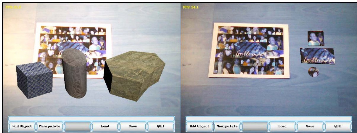
Figure 24: In-situ created objects: Left: Virtual objects textured with predefined textures. Right: Virtual objects textured with textures out of the real world
