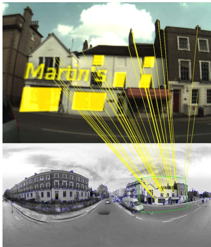
Figure 11 Match of a live image against a stored panorama image and annotations overlaid corresponding to the computed camera pose.
