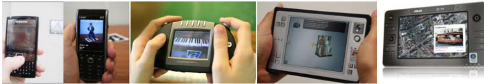
Figure 25: Devices running Studierstube ES range from smartphones and game consoles to ultra-mobile PCs
